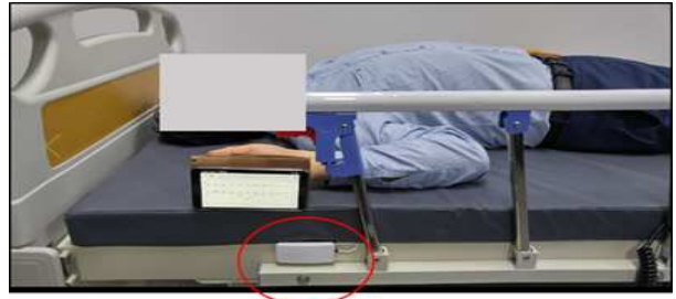
Fig. 2. Hospital bed with BCG sensor
