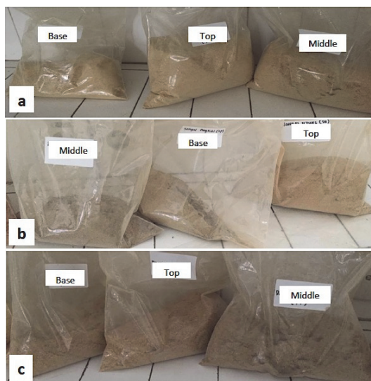
Fig. 2. Samples for chemical analysis of (a) C. melanoxylon ., (b) V. pauciflora , and (c) C. lanceolatum based on log axial direction.
