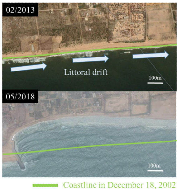
Fig. 10. Severe erosion at yellow boxed area in Fig. 5 due to littoral drift between February 21, 2013 and May 5, 2018.
