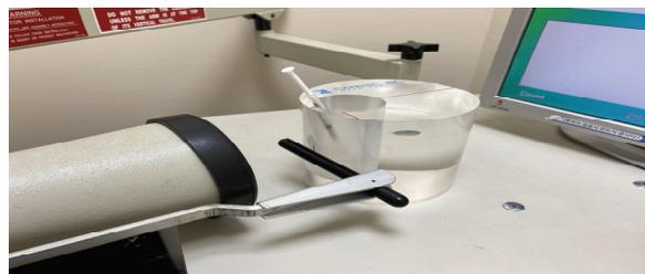
Fig. 2.  $^{99m}\text{TcO}_4^-$  is placed in a syringe and measured for 1 minute using a thyroid uptaker.
