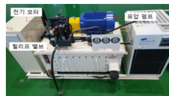
a) Hydraulic Power unit
