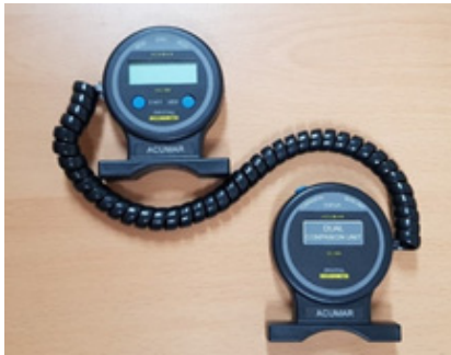
Fig. 2. Dual inclinometer to measure the cervical and lumbar range of motion.
