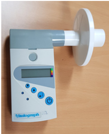
Fig. 1. Vitalograph to measure PEF and FEV1.
