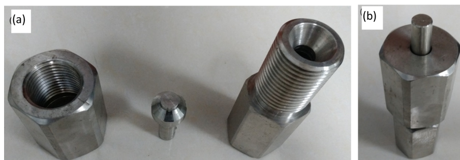
Fig. 1. The photographs of a carbon-silicon composite anode material synthesis device: (a) high pressure reactor disassembly diagram, (b) assembled high pressure reactor.
