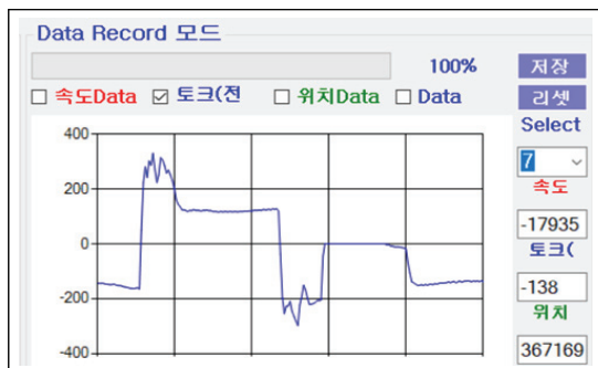
Fig. 14 The torque Control Response of Joint 7
