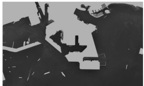
Fig. 7B. Separated Satellite Image by Marker Based Watershed Algorithm
