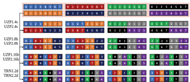
Fig. 3. Register Alignment Structure
