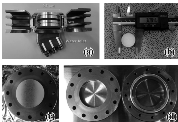
Figure 2. (a) target holder, (b) RbCl pellet, (c) RbCl pellet after beam irradiation, and (d) target cladding with helicoflex seal for ^{82}\text{Sr} production.
