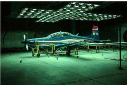
Fig. 2 High Temperature w/Solar Radiation Test
