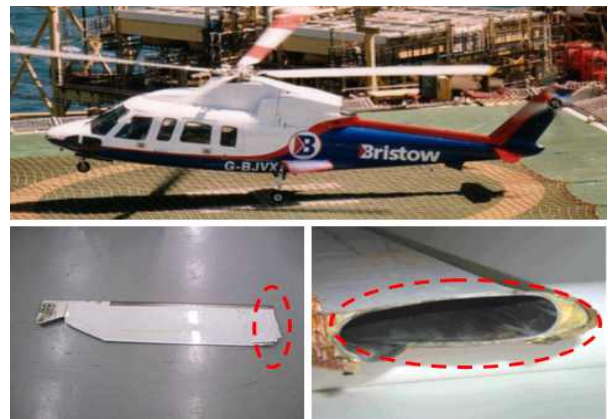
Fig. 1 Lightning strike accident (Sikorsky S-76A+).
