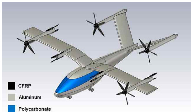
Fig. 7 Model of UAM aircraft implemented in simulation.
