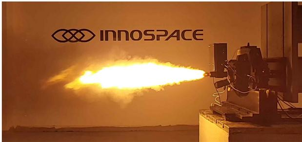
**Fig. 7** Ground Combustion Test of Gas Generator with Control Valve
