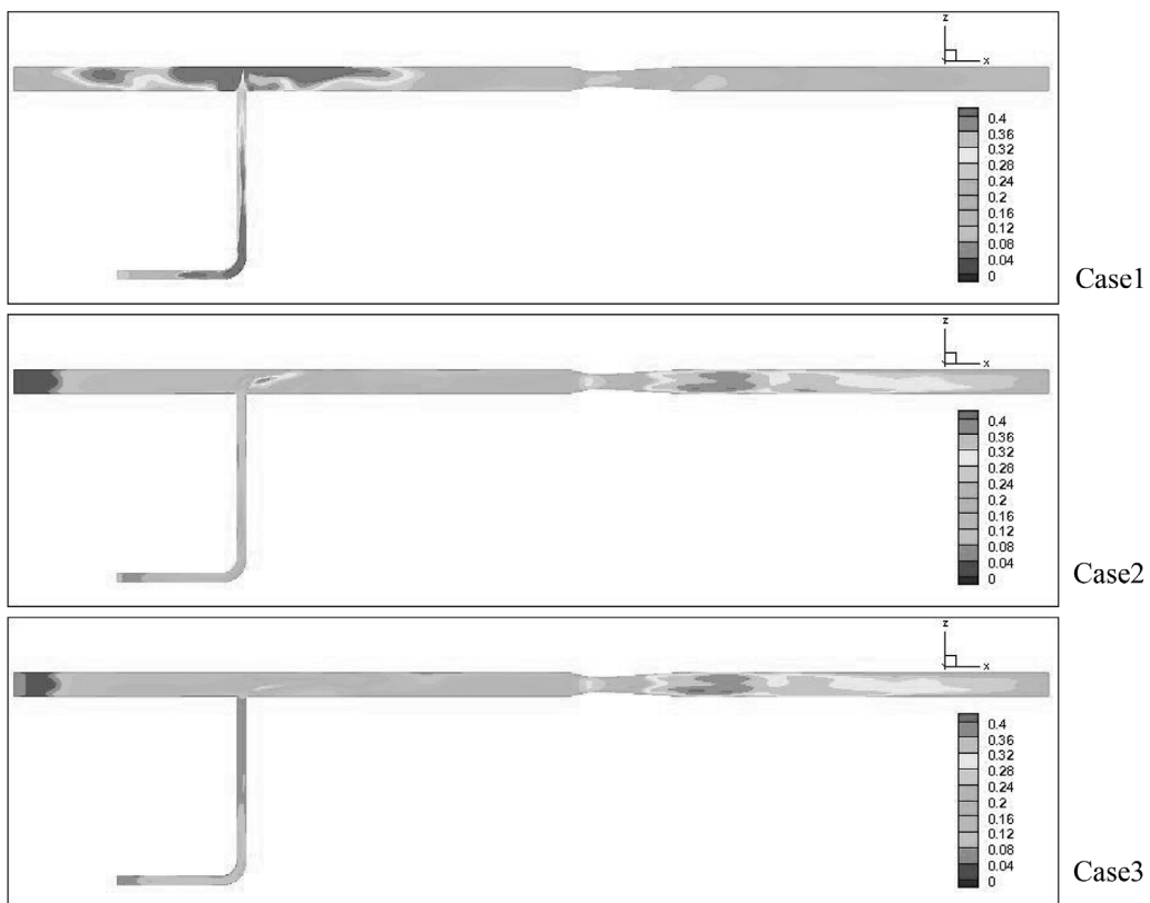
Fig. 7. The contour of the turbulent intensity on the vertical section under different conditions.
