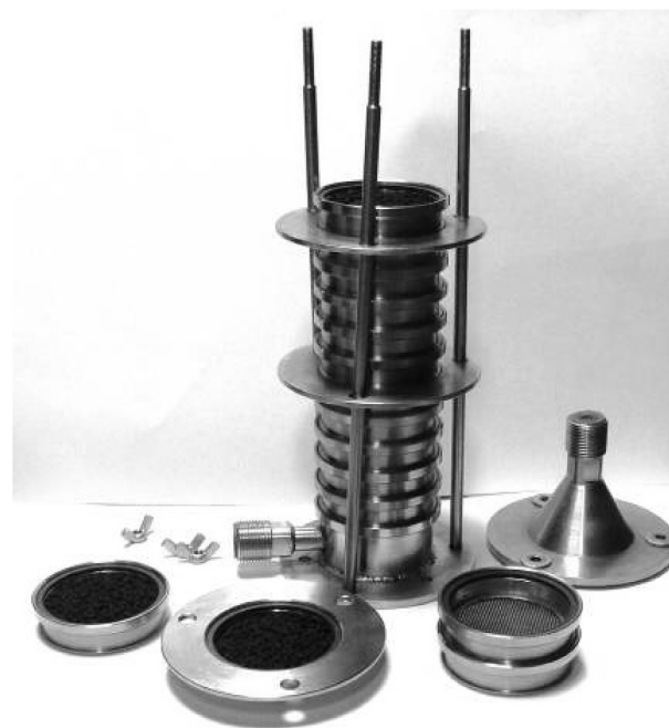
Fig. 1. The layout of the dismountable test column.
