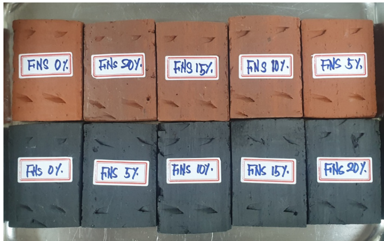
Figure 5. Photo of color change produced by oxidative firing and reduction firing according to the addition of FNS to clay roof tiles
