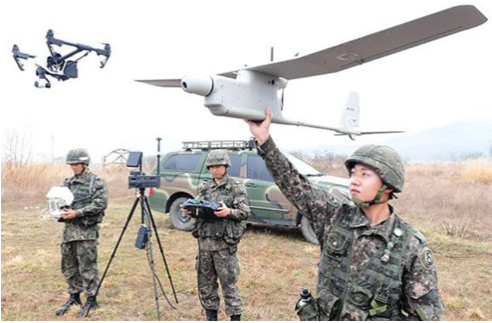
Fig. 1. Operation picture of a hand-launched take-off unmanned aerial vehicle(UAV) in the republic of Korea army(ROKA)
