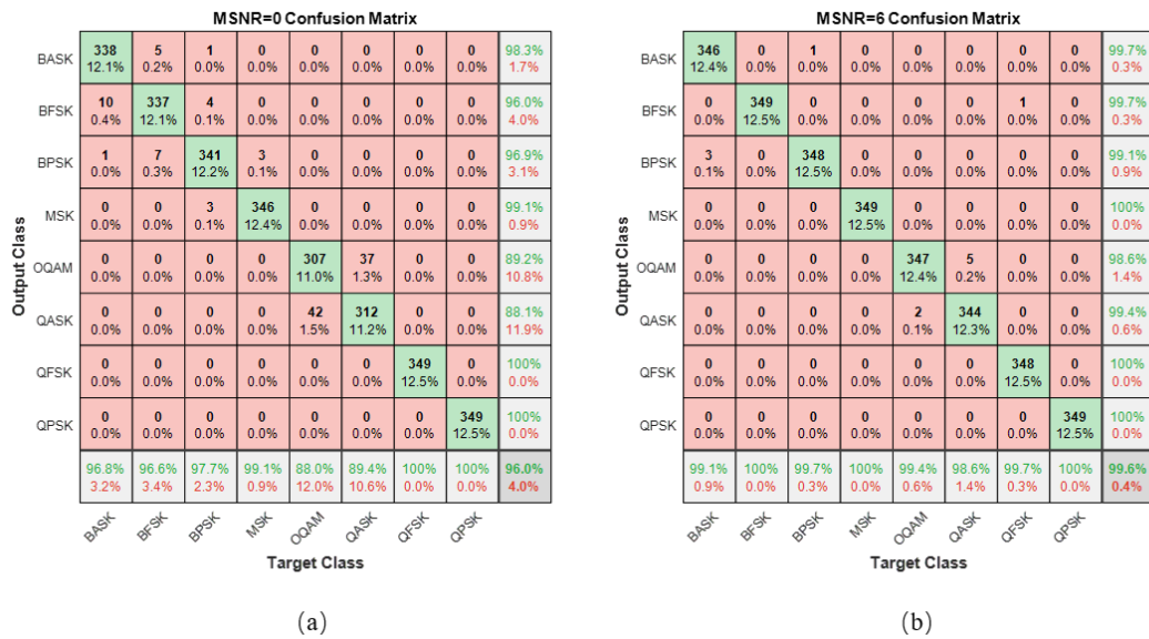
Fig. 5. QEHA-BPNN confusion matrix for the modulation recognition. (a) MSNR = 0dB and (b) MSNR = 6dB.
