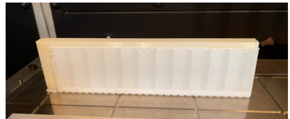
(c) photograph with supports in platform
