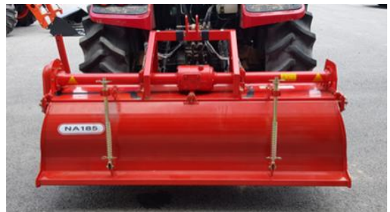
Fig. 2 Forward rotation rotavator
