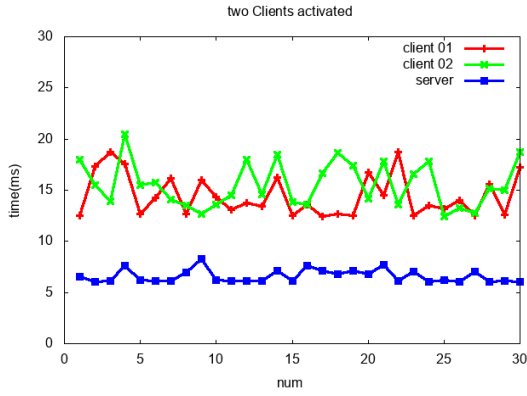
Fig. 8 System background processing when two LiDAR sensor connected
