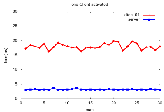
Fig. 7 System background processing when one LiDAR sensor connected
