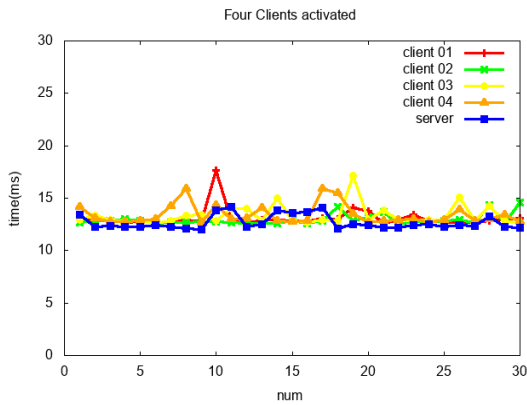
Fig. 10 System background processing when four LiDAR sensor connected
