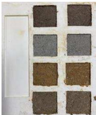
Fig. 6. Making specimen using a framed plasterboard
