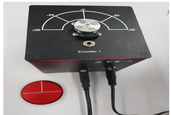
Fig. 2 Rotary motion control testbed: Quanser QUBE Servo 2 system
