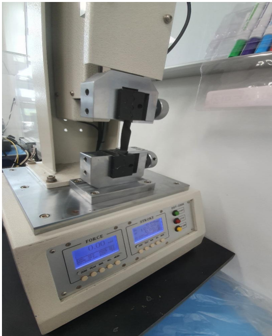
Fig. 4 Elongation test of polyurethane/Carbon Nanofiber Composites
