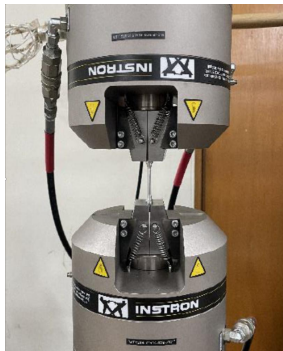
Fig. 7 Photograph of tensile test(Al6061-T6)
