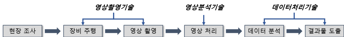
Fig. 7. Process of tunnel inspection using tunnel scanner
