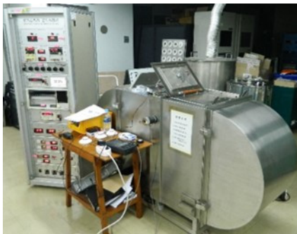
Fig. 3. Measurement apparatus and result of CO sensor installed IoT multi-fire detector
