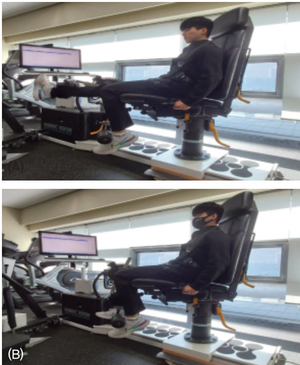
Figure 4. CSNMI muscular strength posture at (A) extension 0° (B) flexion 90°
