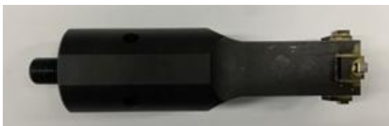
(a) Horn with longitudinal vibration mode
