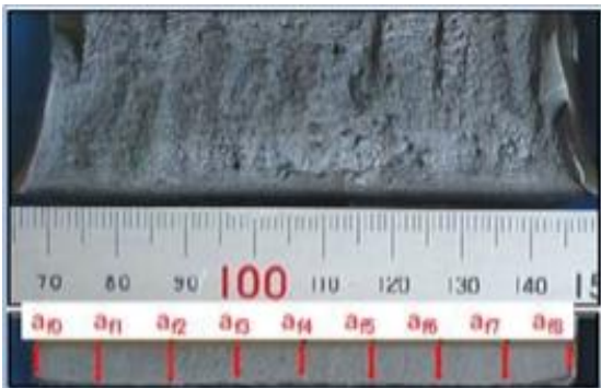
Fig. 2 Location of measuring point for specimen
