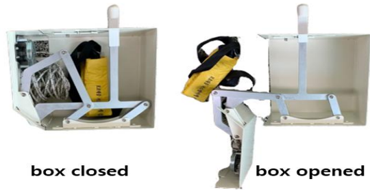
Fig. 10 Operating process for one-touch escape
