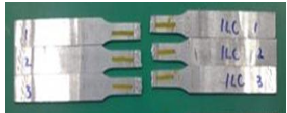
(a) Fracture of weld zone
