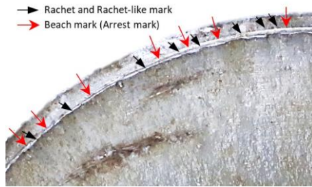
Fig. 5. Detailed fractography of the failed shaft. Oval beach marks, which is barely visible in the photograph, at the multiple points are indicated by the arrow. Ratchet marks at the groove are also shown in the figure.
