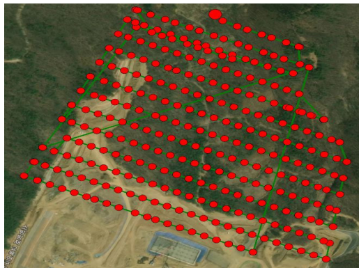
Figure 3. Flight planning and Camera locations
