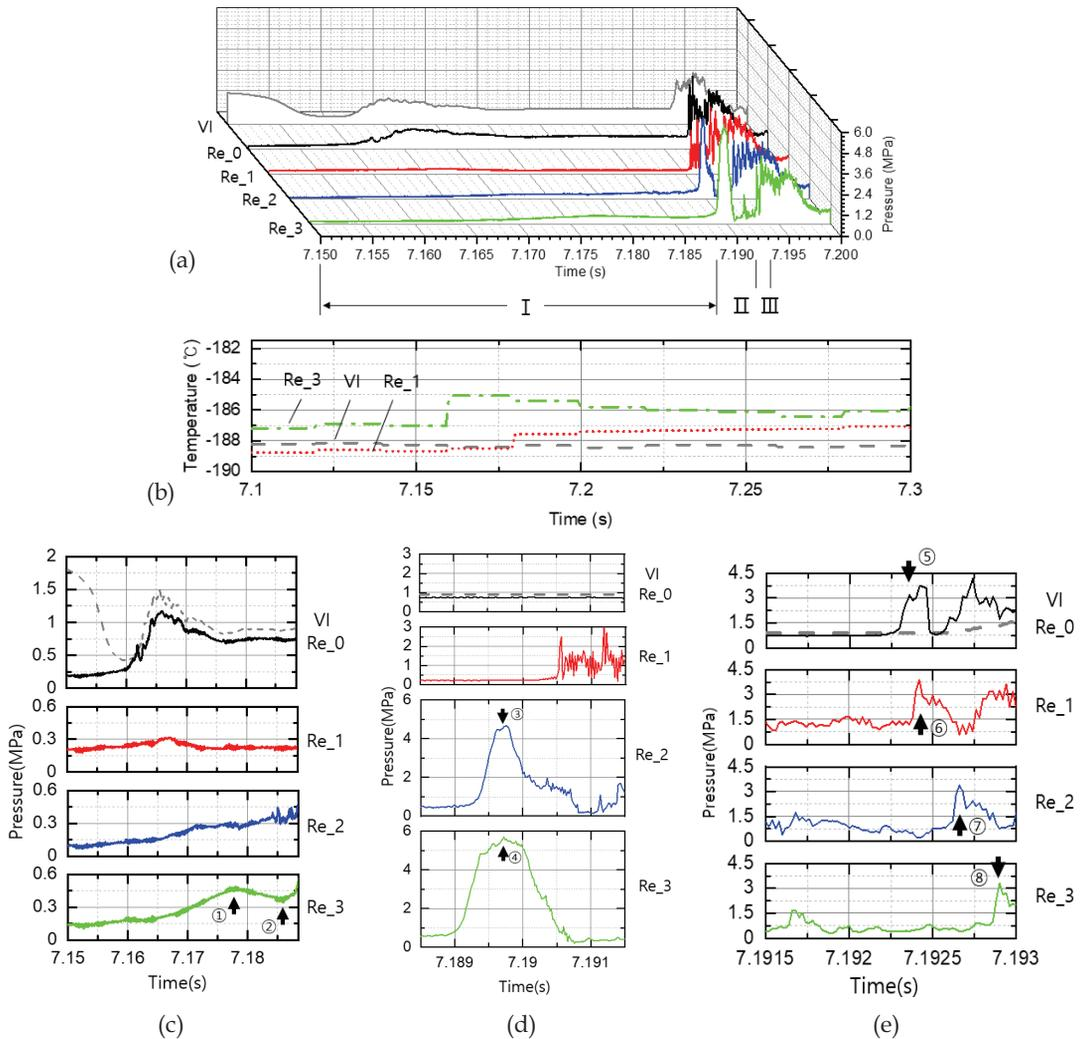
Fig. 6 Experimental results for  $T_0 = -187^\circ\text{C}$  and  $P_0 = 0.212 \text{ MPaA}$  (gray:VI, black:Re-0, red:Re-1, blue:Re-2, green:Re-3), (a) Pressure graph, (b) Temperature graph at each positions(gray-:VI, red-:Re-1, green-:Re-3) (c) Pressure graph at I section, (d) Pressure graph at II section, (e) Pressure graph at III section(-:VI).
