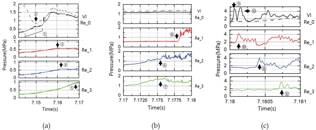
Fig. 5 Experimental results for  $T_0 = -153^\circ\text{C}$  and  $P_0 = 0.287 \text{ MPaA}$  (gray---:VI, black:Re-0, red:Re-1, blue:Re-2, green:Re-3), (a) Pressure graph at I section, (b) Pressure graph at II section, (c) Pressure graph at III section).
