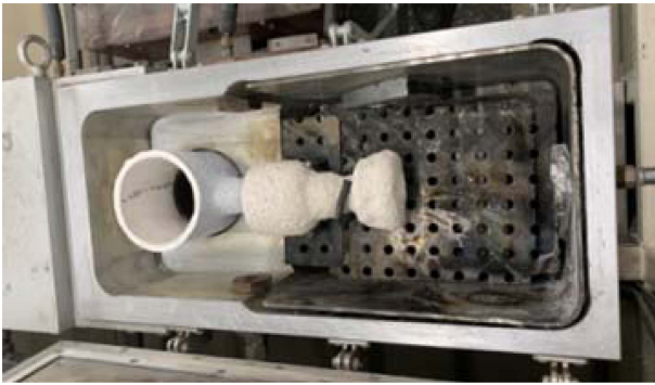
Fig. 1. Vacuum centrifugal casting apparatus for Ti-48Al-2Cr-2Nb alloy.
