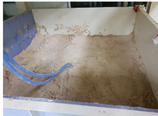
(b) Compaction and injection tube insertion
