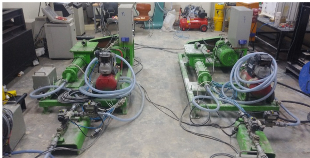
(a) Chemical injection equipment
