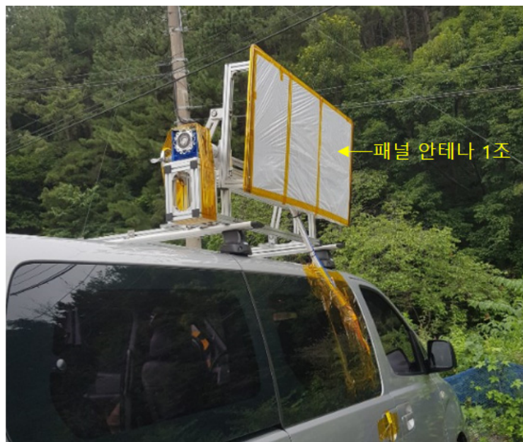
Fig. 3. SAR panel antenna 1 set assembly onboard VAN vehicle for field test. SAR, synthetic aperture radar.
