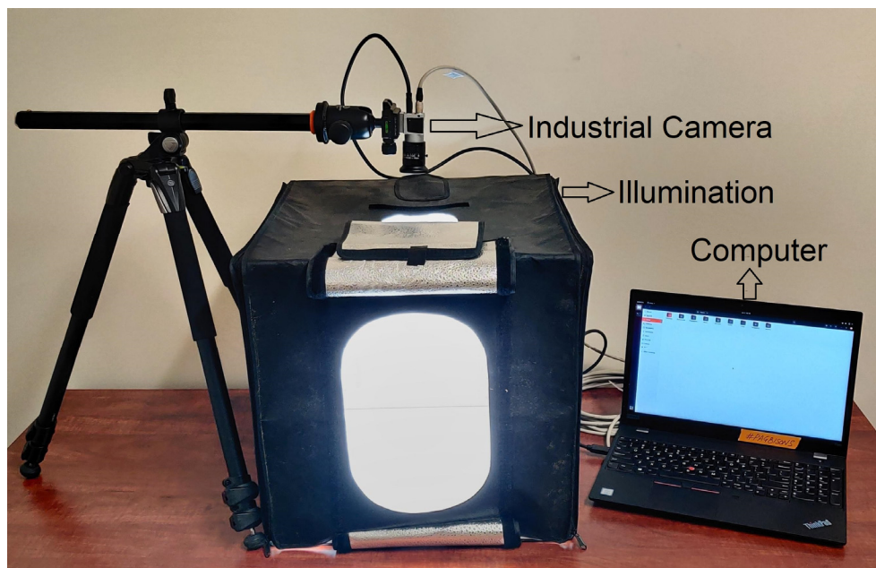
Fig. 1. A typical computer vision system for meat quality non-destructive evaluation applications.
