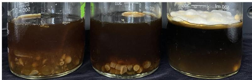
\*left : culture agitated continuously at 120 rpm, center; Culture agitated 1 hr/day at 120 rpm; right, Stationary culture
