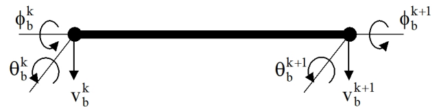
Fig. 4. Degrees of freedom of a beam element
