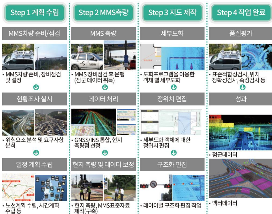
FIGURE 1. Process for generating the precise road maps, captured from a figure in National Geographic Information Institute (2021)
