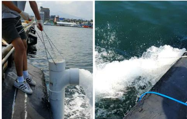
Figure 1. Air-lift experiment at the 10m deep sea water
