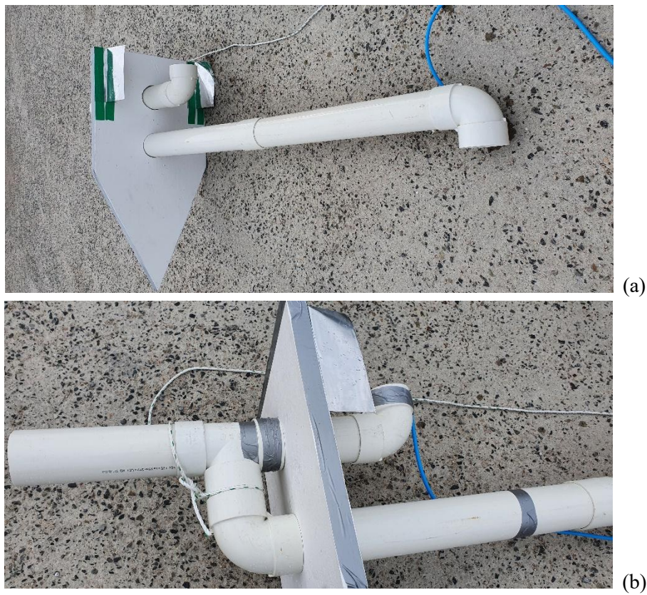
Figure 5. Model ship and propulsion system (a) bottom view (b) side view
