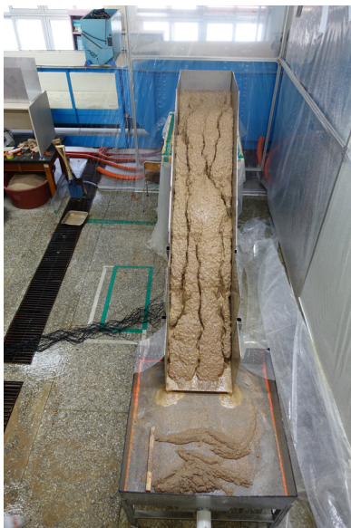
Fig. 4. Rainfall system and soil slope for model test
