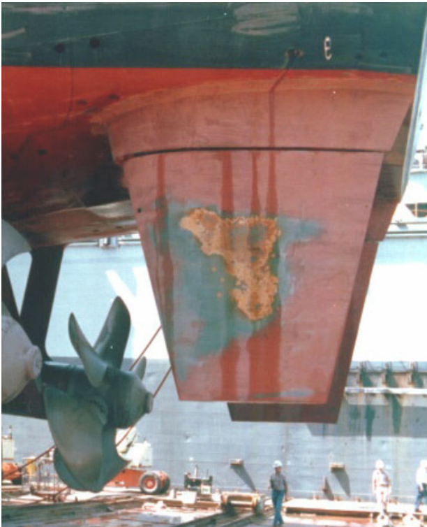
Fig. 2 Example of cavitation erosion in a full-spade rudder
