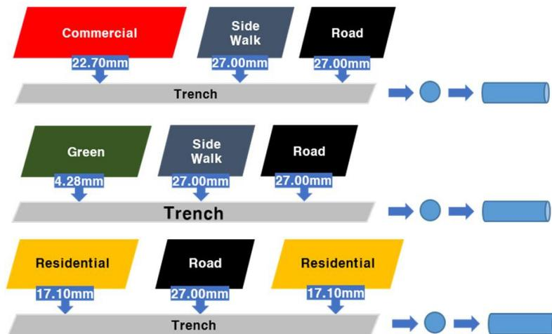
Fig. 4. Depth of Stormwater Runoff by the Land Use
