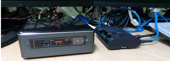
Fig. 3 Performance evaluation testbed with Raspberry PI and Intel NUC
