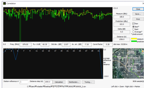
Fig. 9 Comparison between prediction and measurement values at Daejeon city hall area
