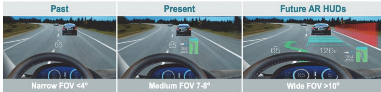
Fig. 1. Future AR-HUDs will allow for a FOV of 10 degrees or more and overlay graphics directly onto the real world (M.Firth 2019)
